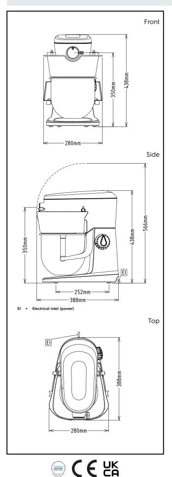
**Electric** 200-240 V/1N ph/50/60 Hz Supply voltage: Total Watts: 0.5 kW Capacity: Performance (up to): 0.75 kg/Cycle Capacity: 5.5 litres
